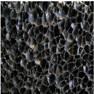
close-up, enlarged picture of noise absorbing material
